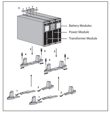
Use the same procedure for tower mounting multiple battery modules, if applicable.
